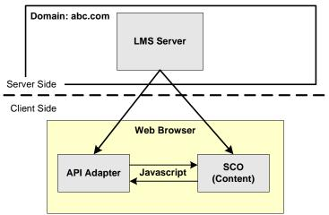
Figure 3.1a – One LMS/Content server with no virtual IP addresses
